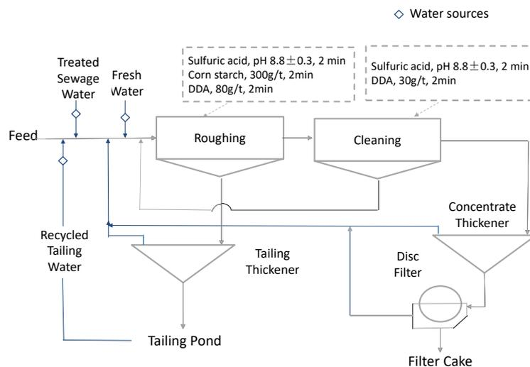
Fig. 2. The flowsheet of an industrial flotation plant of iron ores in Yunnan Mine
