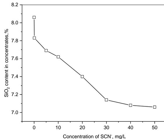
Fig. 9. Effects of  $\text{SCN}^-$  ions pre-treating the tailing water on the content of  $\text{SiO}_2$  in concentrates
