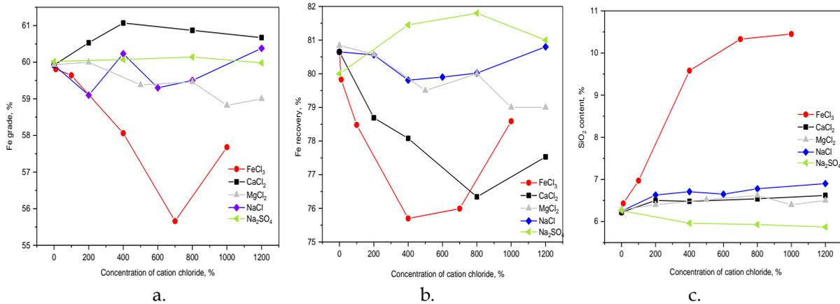
Fig. 5. Grade Fe (a), Recovery of Fe (b), and content of SiO<sub>2</sub> (c) in concentrates as a function of cation chloride or sodium sulfate concentrations at a pH range of 8.7±0.2
