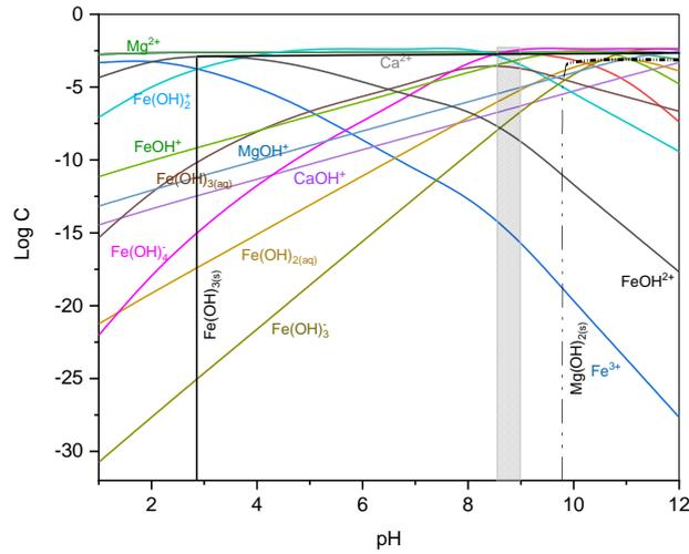
Fig. 7. Log C-pH curves of cations, such as  $\text{Ca}^{2+}$ ,  $\text{Mg}^{2+}$ ,  $\text{Fe}^{3+}$ , and  $\text{Fe}^{2+}$  at a concentration of 5 mmol/L in water
