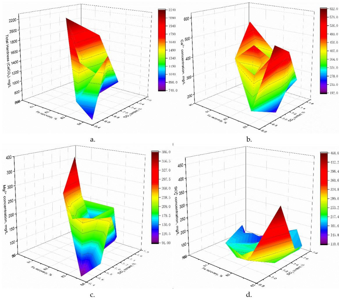
Fig. 4. The records of ion distributions in the process water from the roughing stage on the Fe recovery or SiO<sub>2</sub> content in concentrates in the industrial iron ore flotation plant at a period from June, 1st to August, 1st, 2021 ((a. total hardness, b. Ca<sup>2+</sup>, c. Mg<sup>2+</sup>, or d. SO<sub>4</sub><sup>2-</sup>)
