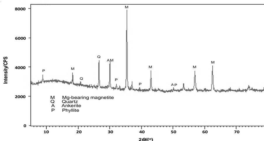
Fig. 1. XRD analyses of the iron ore sample from Yunnan Mine, China
