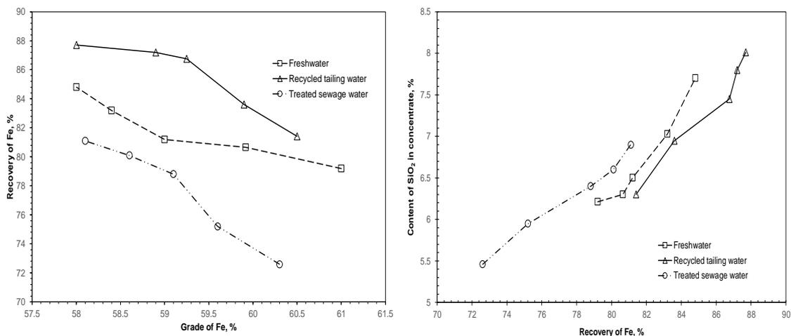
Fig. 3. Flotation performance (a. Grade of Fe vs recovery of Fe, and b. content of  $\text{SiO}_2$  vs recovery of Fe) of the iron ore by using different water sources at a pH range of  $8.7 \pm 0.2$
