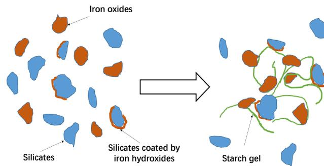
Fig. 10. The possible depression mechanism of  $\text{Fe}^{3+}$  on the quartz floatability in the presence of starch
