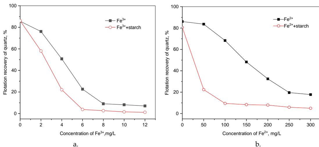
Fig. 8. Recovery of quartz as a function of  $\text{Fe}^{n+}$  ion concentrations with or without 4 mg/L starch at  $8.7 \pm 0.2$  (a.  $\text{Fe}^{3+}$ , or b.  $\text{Fe}^{2+}$ )
